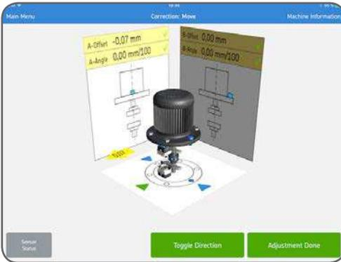
Alignment is now complete and to confirm the result there is a need to re-do the measurement. Tap Remeasure.
