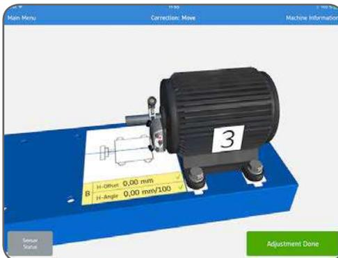
An animation shows the bolts being tightened down. Alignment is now complete and to confirm the result there is a need to re-do the measurement.
