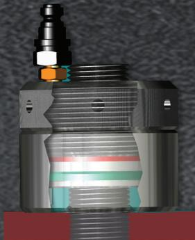
Assemble the Hydraulic Nut onto the bolt to be tensioned.
