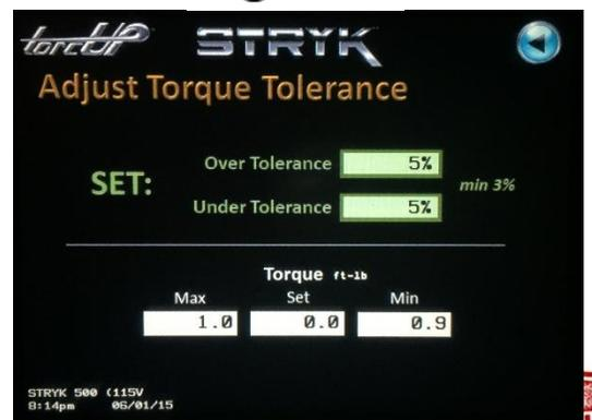
3. Set desired tolerance for the PREVAILING TORQUE, by touching the OVER TOLERANCE and UNDER TOLERANCE fields and using the drop down keypad to enter the percentage tolerance. The minimum and maximum torque values will be displayed. (See Figure 8)
