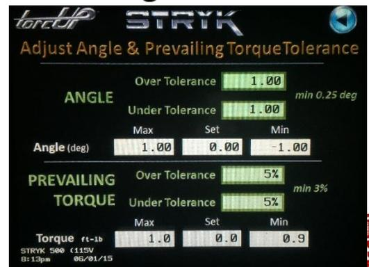
After all data has been input, press RUN to operate the STRYK tool. The tool will tighten to the set prevailing torque.
