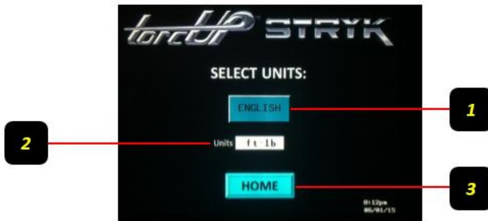
The UNITS screen currently offers two selections. At this time, the STRYK has the capability to display in imperial and metric units.
