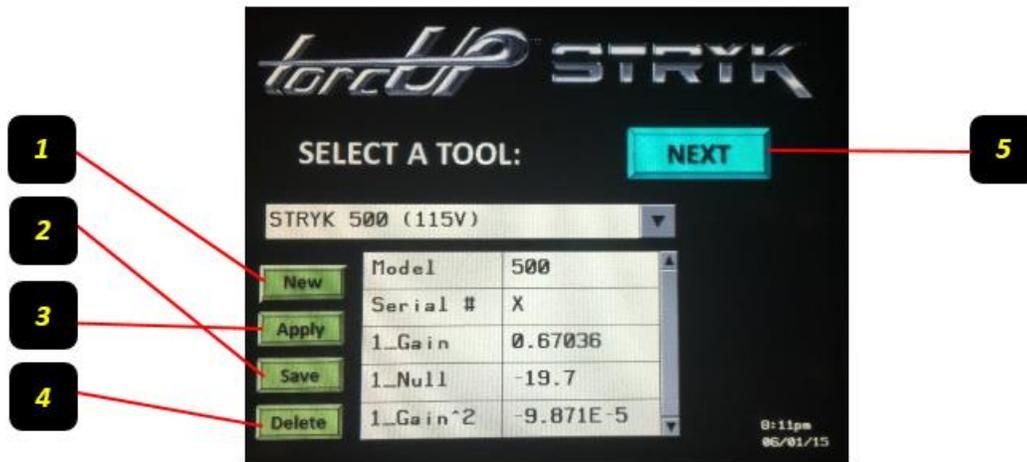
1. **NEW** – is used to enter a new tool. Touch the NEW button, and a new model number will appear. This tool model can be changed to a name of your choice by touching field tool selection field to the right and using the drop down keypad to enter desired tool name. Press ENTER when complete.
