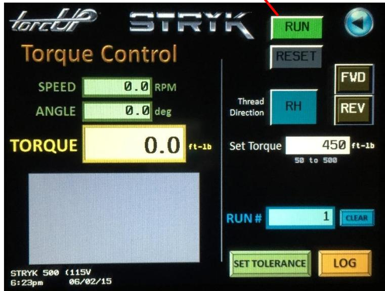
Each time the tool is operated, the indicator will flash either PASS or FAIL on the readout section of the control screen. The LED indicator on the rear of the tool handle will also show an indication of pass or fail, giving the operator a visual indicator without having to examine the control box.
