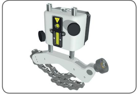
Use the extension chain for shafts  $> \varnothing 150$  mm ( $> \varnothing 6.0$  inch).
