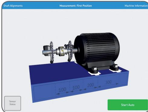
*When the system senses that the shaft has been rotated sufficiently, and has been left untouched for a short while, it will automatically record the 2<sup>nd</sup> measurement position.*
