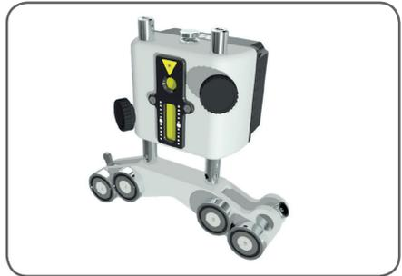
Align both fixtures tangentially on the coupling by using the shaft brackets, or the magnetic surface of the magnets.
