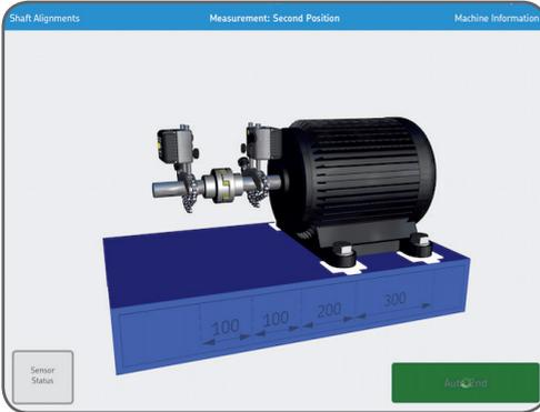
*When the system senses that the shaft has again been rotated sufficiently, and has been left untouched for a short while, it will automatically record the 3<sup>rd</sup> measurement position.*
