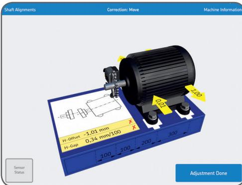
After the correction, or if no correction is needed, tap Adjustment Done.
