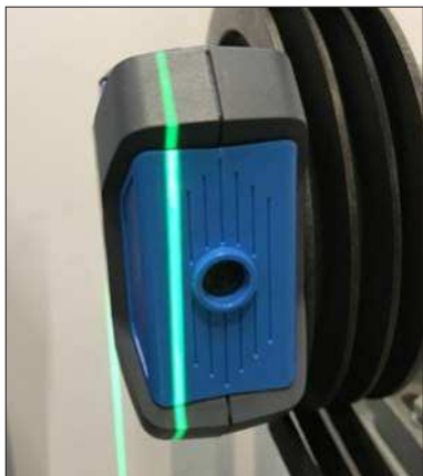
Fig.7 – Display of parallel misalignment (offset)
