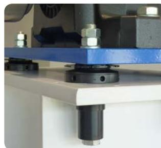
SKF Vibracon solution for resilient mounts
