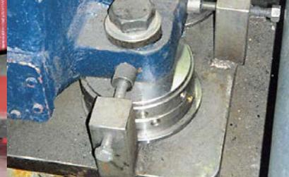
Intermediate shaft bearing Skid mounted diesel engine
