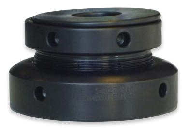
For applications where the combination of space versus strength becomes critical, SKF developed a special heavy duty chock. In addition to a higher load capability, also the adjustment range has been extended. This makes the SKF Vibracon – heavy duty, the ultimate adjustable chock solution for industrial applications. Common applications are, for example; compressors, pumps, steam and gas turbines.
